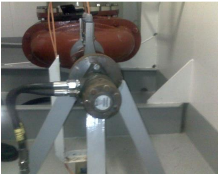
Figure 20 Example of a typical installation of Hydraulic motor
